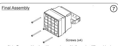
Note: Ensure cables do not become trapped in the casing. When wiring is completed, mount front of Mosquito Sounder onto the back box and fix using the screws provided.
